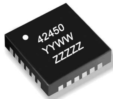
Figure 2. Package Photo 24-lead 4x4x0.85 mm QFN Package
